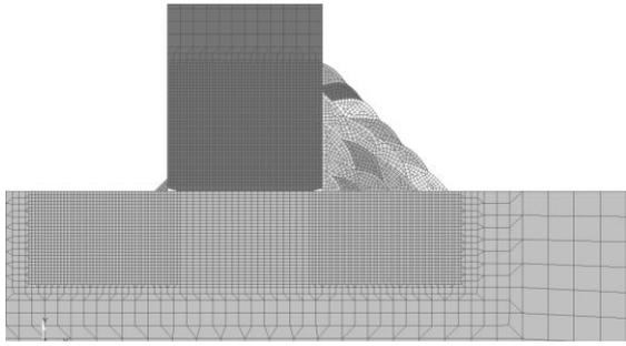
Fig. 3: Discretization of a multistage welding process of a T-joint.
