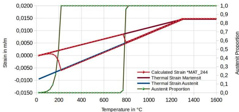
Fig. 10: Curve of strain vs. temperature for a dual-phase steel.
