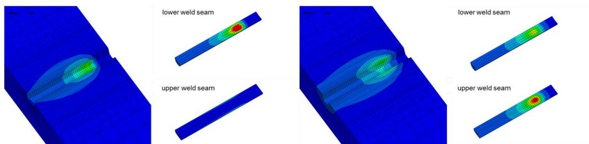
Fig 7: Temperature distribution in round robin example at  $t=9.6$  (left) and  $t=28$  (right). Shown temperature ranges between room temperature and 1900 K.
