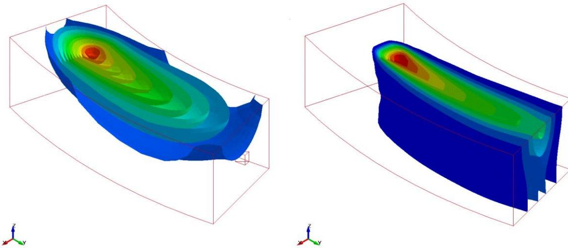
Fig. 2: Temperature iso-surfaces for a Goldak double ellipsoidal (left) and a double cone-shaped (right) heat source. Both defined in LS-DYNA using an analytical expression.
