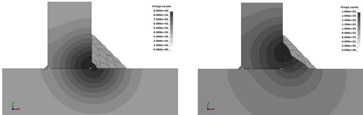
Fig. 4: Temperature distribution during a multistage welding process after the first stage (left) and after the ninth stage (right).
