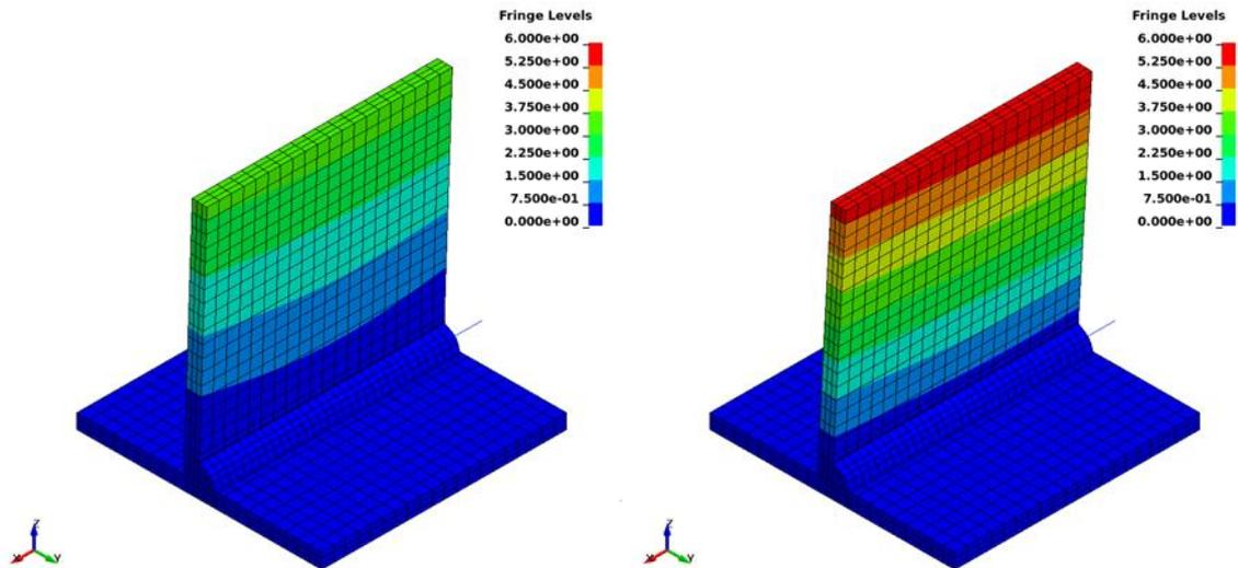
Fig. 5: Comparison of the displacement field after the completed welding process. On the left, all material is activated at the beginning, on the right, ghost material is used as filler material.
