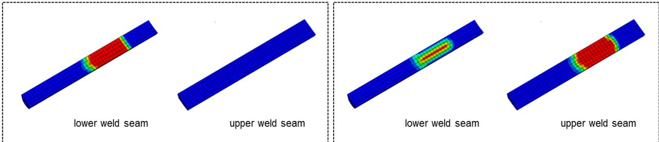
Fig. 8: Austenite concentration at t=9.6 (left) and t=28 (right).
