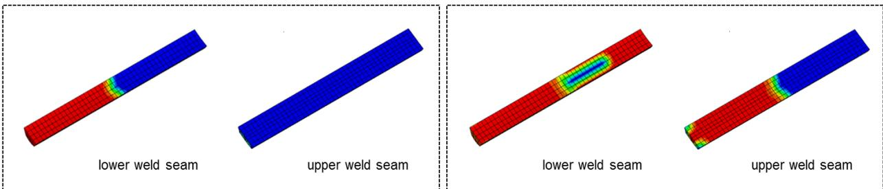
Fig. 9: Martensite concentration at t=9.6 (left) and t=28 (right).
