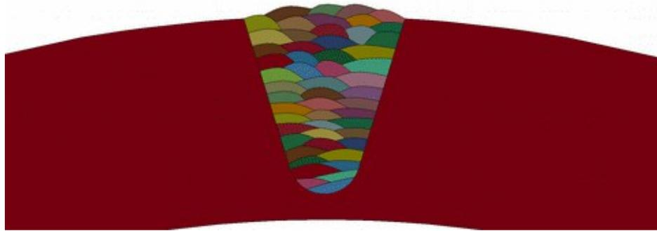
Fig.11: Cross section with 53 passes SAW
