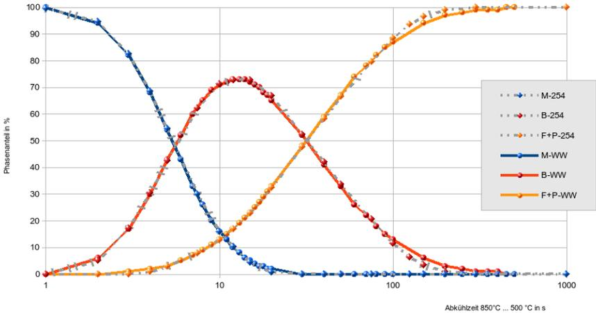
Fig 1: S420 Phase Proportion calculated with \*MAT\_254 compared with given data
